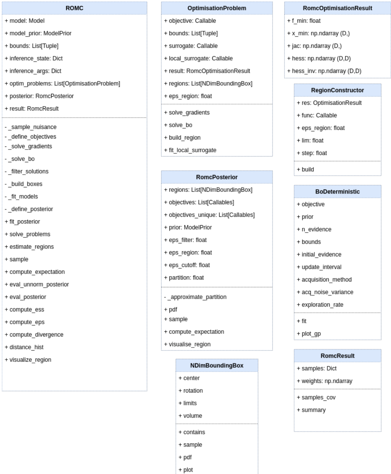
Figure 8: Overview of the entities (classes) used at the deployment of the ROMC inference method, at the ELFI package.
